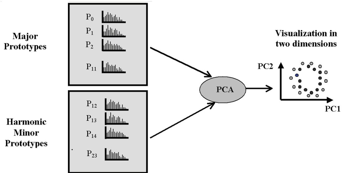
*Figure 1.1.* Projections of prototypes are displayed on the first two principal components.
